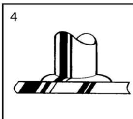
4 The weld gun is withdrawn from the weld stud leaving the weld and the ferrule. The ferrule is broken away and discarded. Visually inspect weld.
