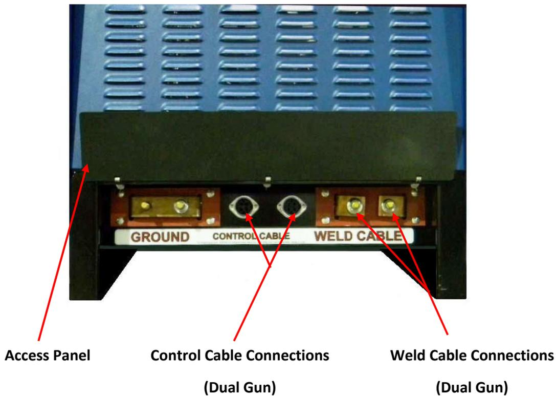
After the cables are connected to the welder, it is time to configure your weld gun for its specific job. Once the gun is configured and set up properly, the gun cables will connect to the weld cables. For the SC2420, the weld cable ends that connects to the Heavy-Duty TWE17000 Stud Gun will be a female Control Cable Plug and a female Heavy-Duty High Temperature camlock connector.
