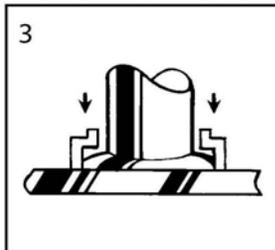
3 The main spring plunges the weld stud down into the molten pool of metal in the base material. The cycle is completed in less than a second and the resulting weld bond develops the full strength of the fastener in the weld zone. Allow metal to cool and withdraw gun from the stud, pulling the gun straight up off of the stud.
