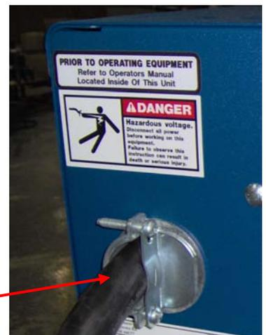
Route primary power cable through power inlet hole and tighten down clamp.
